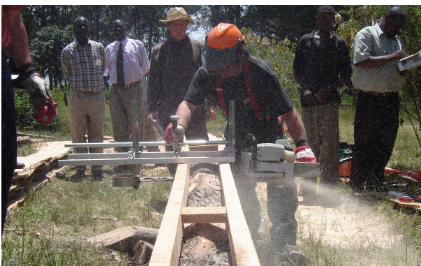
The first cut with a frame mill and homemade 'slabbing rails'. The first 'Alaskan'-sawn Grevillea in Kenya
