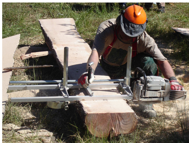
Chainsaw milling with an Alaskan frame mill in Kenya.
