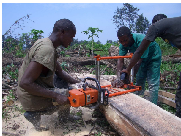
Using a chainsaw frame mill in DR Congo.
