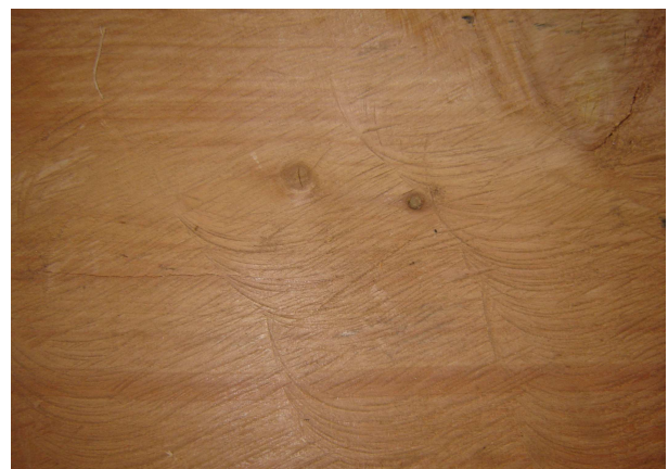
The tell-tale 'trademark' of freehand chainsaw milled timber. Khaya spp. in Kenya, illegally harvested.
