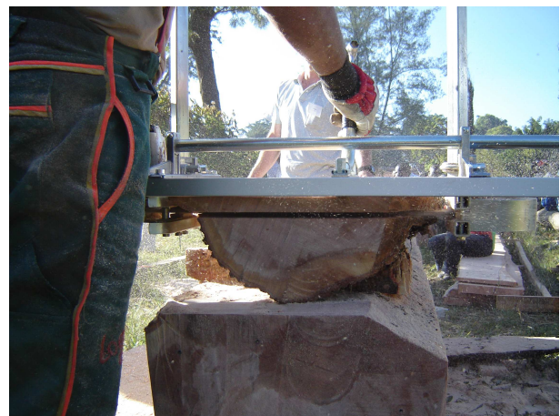
Using a frame mill to cut extra boards from a side slab that would otherwise have been firewood.
