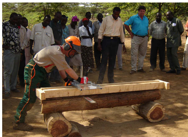
Chainsaw milling Prosopis juliflora, a dryland weed in Kenya. Note homemade 'slabbing rails' for the first cut.
